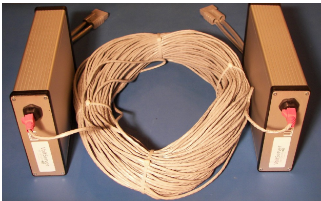
Figure 5: PET Transmitter/Receiver shown with 100m of CAT-5 Cable
